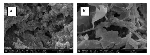
For the CAC composition (Figure 2.a), it is possible to observe the presence of countless needled crystals, resulting from the CAC hydration process and responsible for providing green mechanical strength to the sample. When observing the microstructure of the Fastfrax®-bonded castable (2.b)), it is possible to notice a completely different structure, where an interconnected gel structure is formed throughout the material, with the
