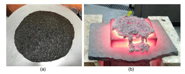
Figure 1 - (a) Self-flow test for self-flow repair mix; (b) Thermal flow at 1,000°C.
