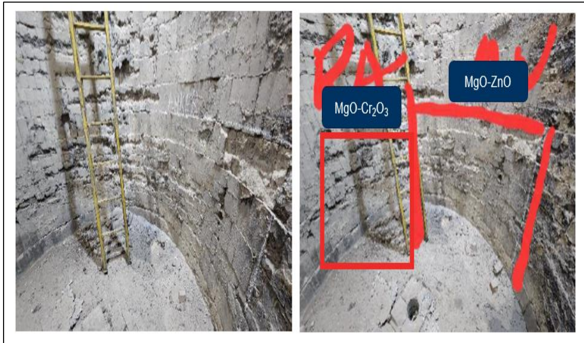
Figure 2. MgO-Cr 2 O 3 and MgO-ZnO after trial (40 heats).
