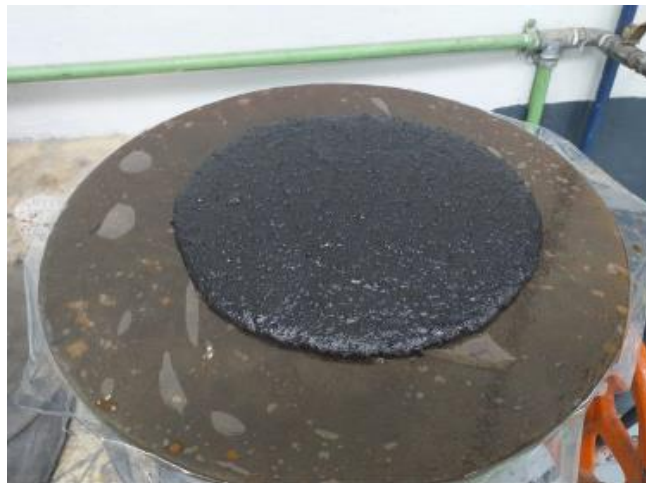
Figure 1: Self-flow test for quality control of MgO-C castable.
