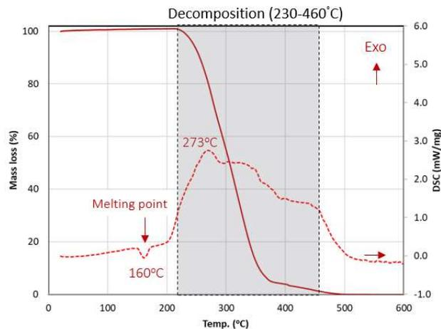
Fig. 9 Mass loss (%) and DSC (mW/mg) of Fibre-P1 during heat up.
