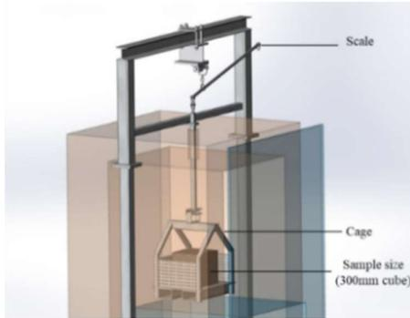
Fig. 2: Illustration of the industrial-scale thermo-balance (Macro-TGA)
