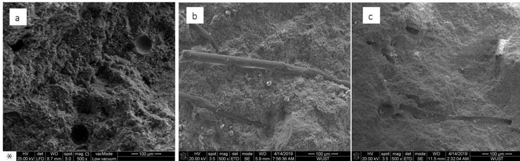
Fig.11: SEM of fractured surface of NCC samples heated at 120°C for 12hrs. a) NCC REF, b) NCC with Fibre-P1, and c) NCC with EMSIL-DRY™.
