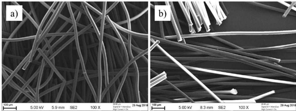
Fig. 10 SEM image of drying agents. a) EMSIL-DRY™ and b) Fibre-P1.
