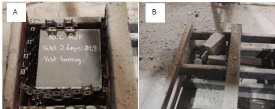
*Fig.5: ~80kg block (A) before and (B) after explosion resistance test (from 20 to 850°C at 50°C/hr).*
