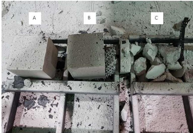
*Fig.6: ~80kg (300mm) cubes with different fibres after explosion resistance test (from 20 to 850°C at 50°C/hr). A) Fibre P3, B) EMSIL-DRY™ and C) Fibre-P1. The NCC with Fibre-P2 looked like cube C) Fibre-P1.*
