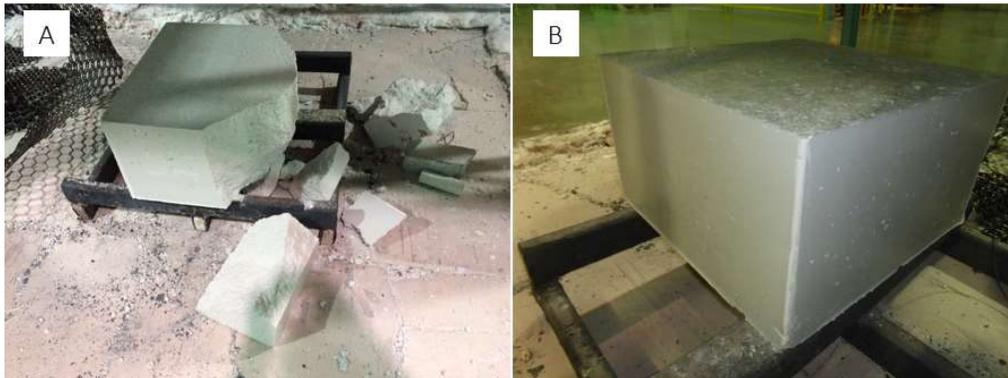
*Fig.7: ~400kg blocks after explosion testing at 850°C. A) Fibre-P3 and B) EMSIL-DRY™*
