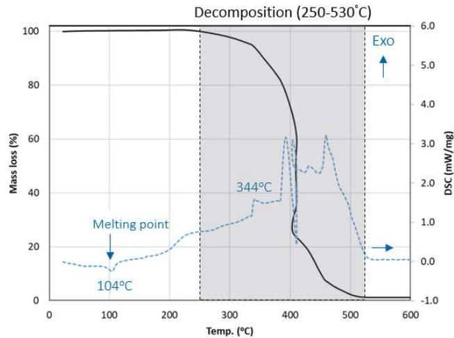
Fig. 8 Mass loss (%) and DSC (mW/mg) of EMSIL-DRY™ during heat up.
