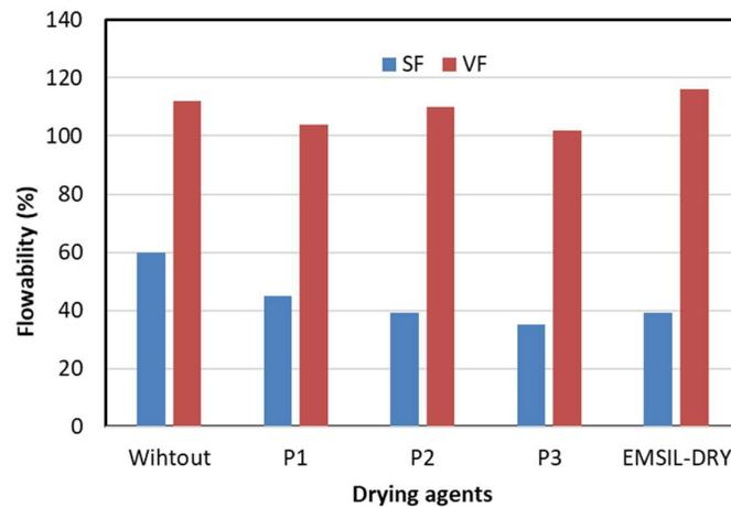
Fig. 4: Flowability of microsilia-gel bonded NCCs with different drying agents.
