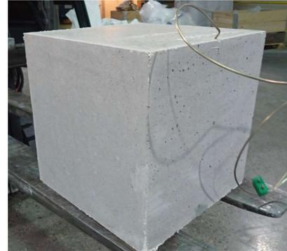
Fig.3 and 300mm cube with embedded thermocouple in the centre
