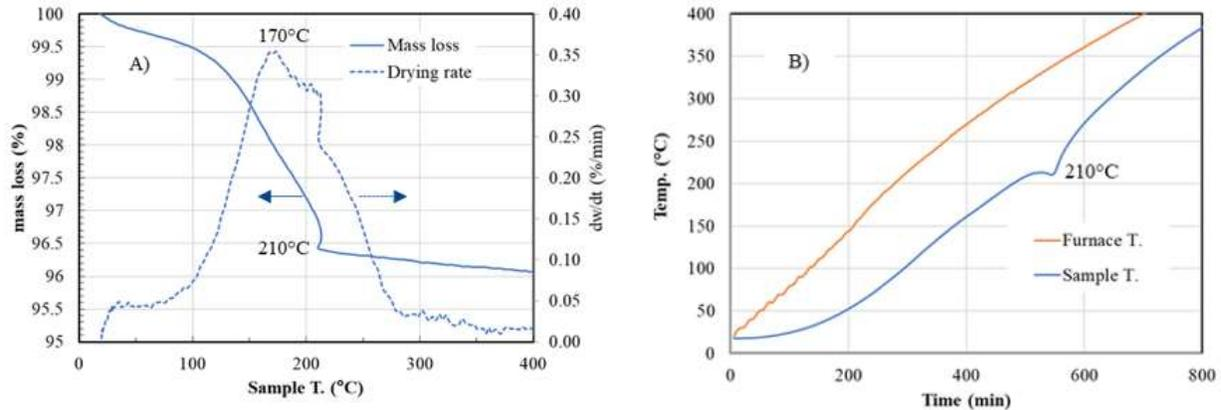
Fig. 12: Drying behaviour of NCC containing EMSIL-DRY™ using Macro-TGA. a) Mass loss (%) and Drying rate ( $dW/dt$ ), and b) Furnace temperature and sample temperature.
